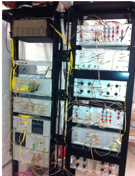
Equipment combines the 12 different carrier signals into one composite signal.
